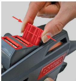
Figure 22 Compressing springs of cliché-slide
