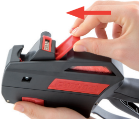
Figure 22 Push the cliché-slide forward
