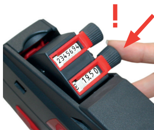
Figure 8 Pushing back adjustment knob
