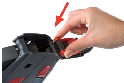
Figure 15 Inserting ink roll
